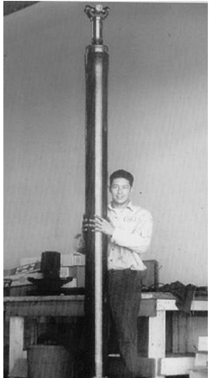
Figure 2-2: One Piece Carbon Fiber Driveshaft, Garbage Truck Application
