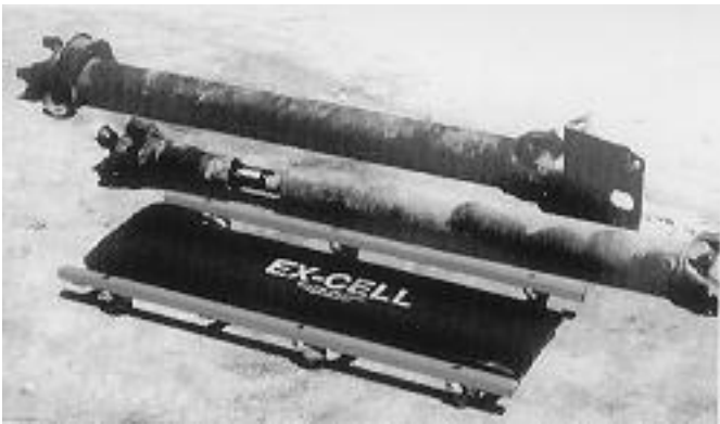
Figure 2-3: Two Piece Steel Shaft, with Center Bearings, Removed from Garbage Truck
