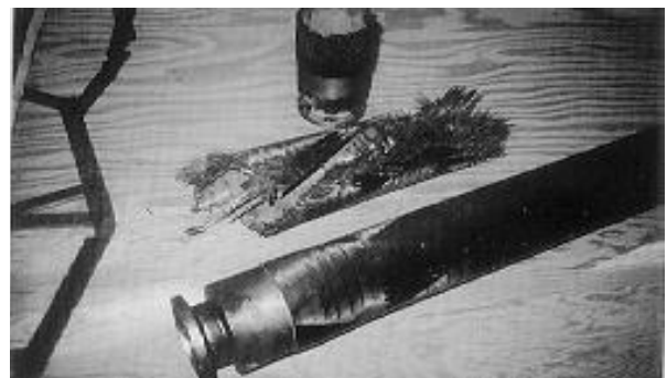
Figure 5.1 Carbon Fiber Driveshaft: Energy Absorbing Break
