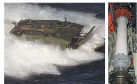
Left & Right: ACPT custom composite couplings were employed in the carbon composite powertrain for the Marine Expeditionary Fighting Vehicle (EFV), shown here on maneuvers in the desert and at sea preparing for a beachhead landing.
